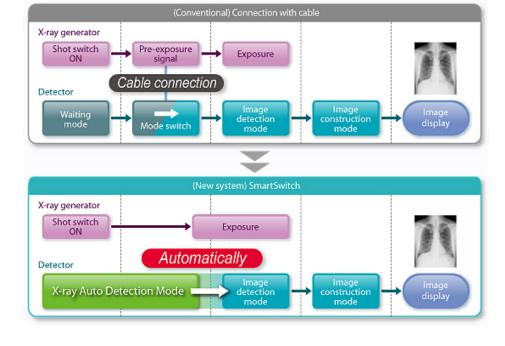
Fast imaging — rapid display of images and automatic trimming ensure smooth examinations
